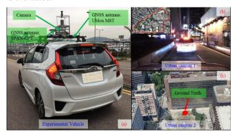
**Fig. 4** The sensor setup of the experimental vehicle and evaluated scenarios. (a) sensor setup of the experimental vehicle. (b) the experimental scene with tall buildings in urban canyon 1. (c) the experimental scene in urban canyon 2.
